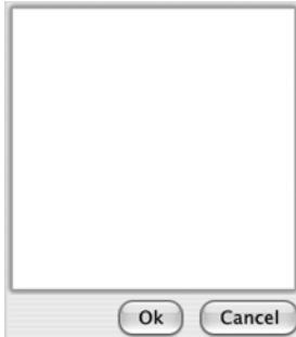
Figure 6.7 A FormLayout has been used to position the two buttons relative to the text area.
